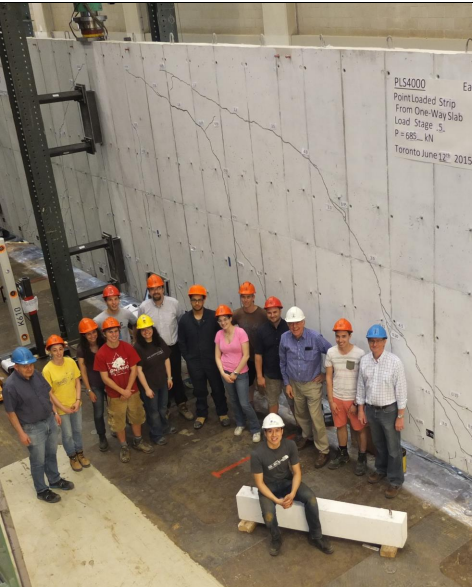
Test of a 4 m deep reinforced concrete slab strip at the University of Toronto in 2015. This remains the largest reinforced concrete shear test ever performed.
