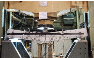
Fig. 33.2 – A reinforced concrete beam tested by Garratt et al. which failed in flexure. Note the large cracks and displacements, as well as the crushed concrete at the top of the beam.
