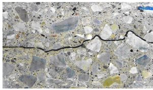
Fig. 34.3 – Interlocking of aggregate in a concrete member, preventing sliding along the crack.
