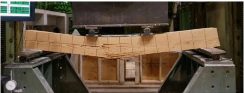
Fig. 26.4 – Timber beam loaded under four-point bending. Note the shear failure on the left side of the beam which has caused the previously vertical lines to separate, and the flexural failure at the midspan.
